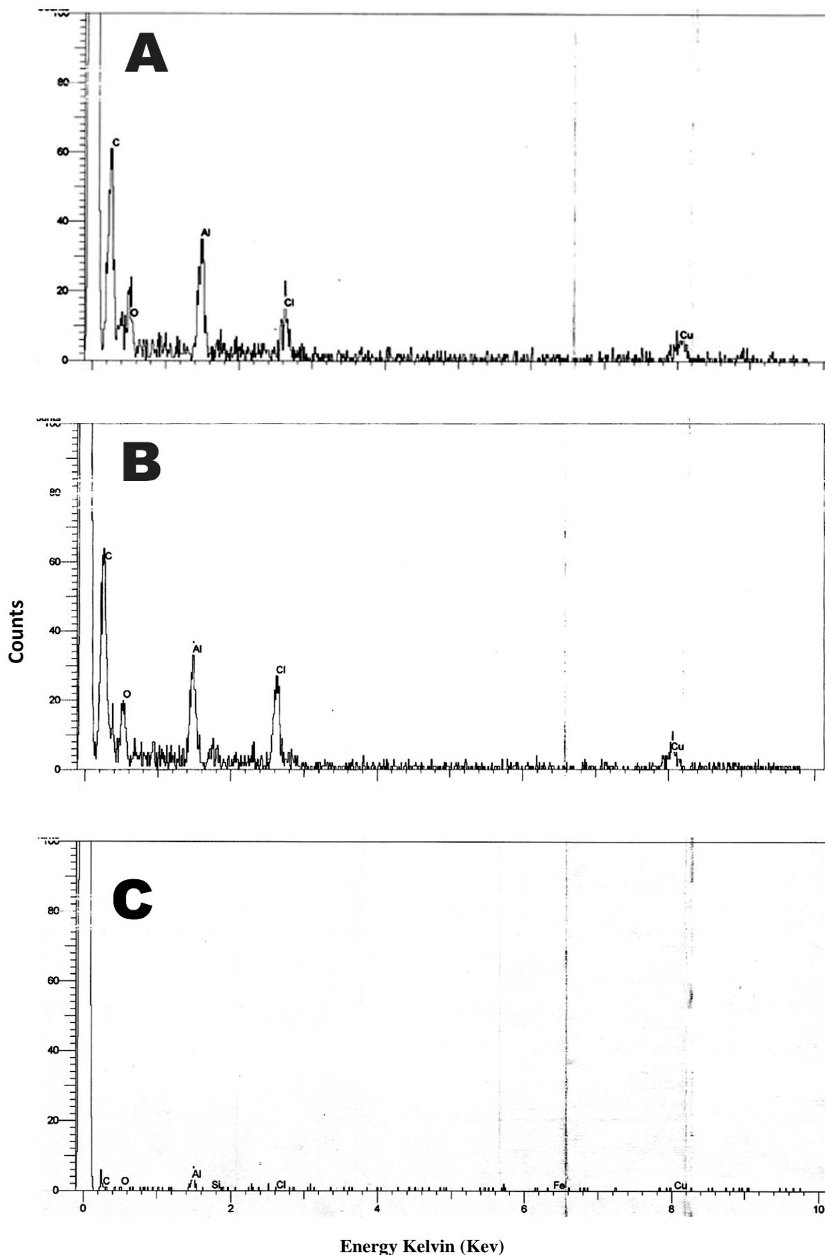
Fig. 2A. Energy Dispersive x- ray Analysis of electron opaque materials CMG462 grown in presence of copper sulphate. A, analysis inside the cells, B, analysis at cell surface and C, control.
